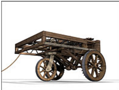
A replica of da Vinci’s vehicle with programmable steering; the rope acts as a remote control to release the brake, whereupon the wagon travels up to 40 meters. Illustration by the da Vinci Museum.
