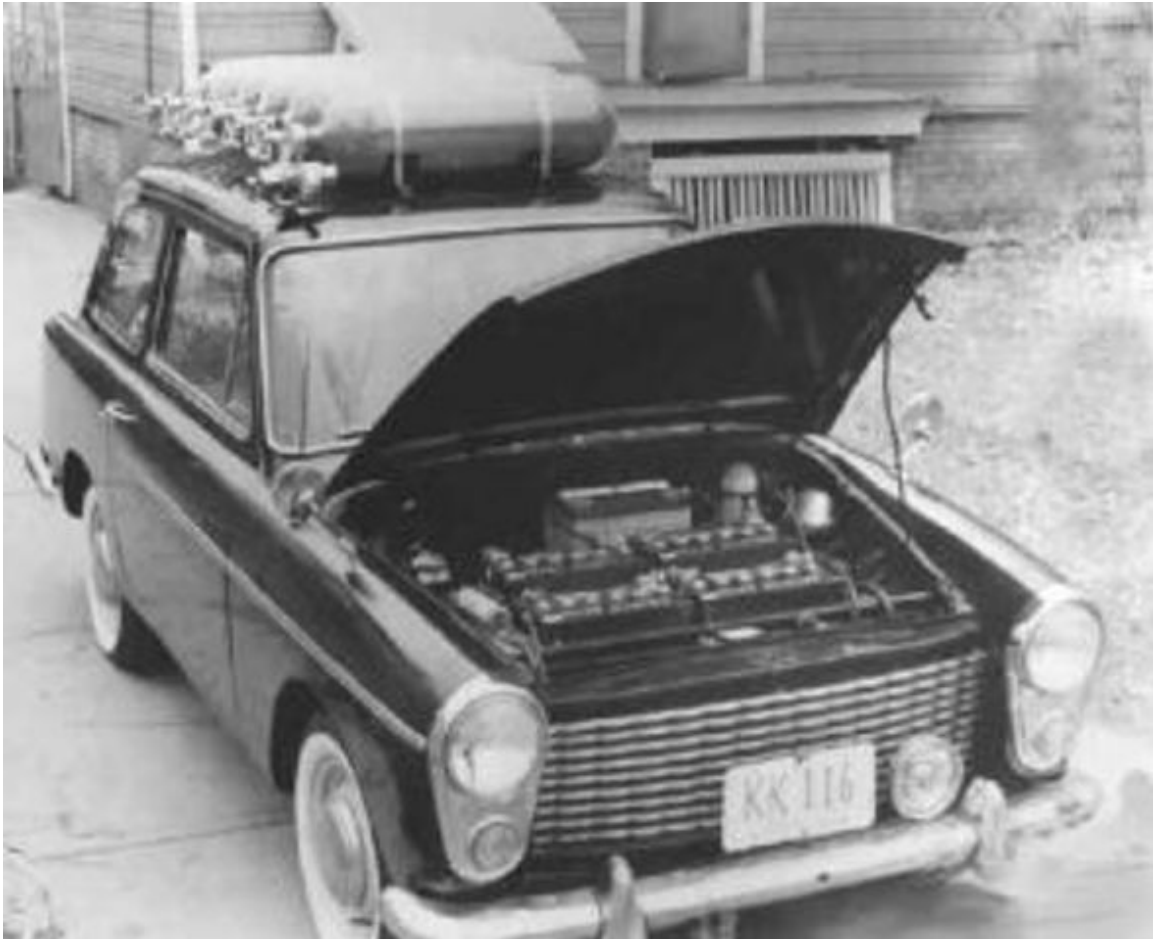
A battery of batteries under the bonnet (hood) of the Austin A40. Illustration courtesy of the Union Carbide Corporation.
