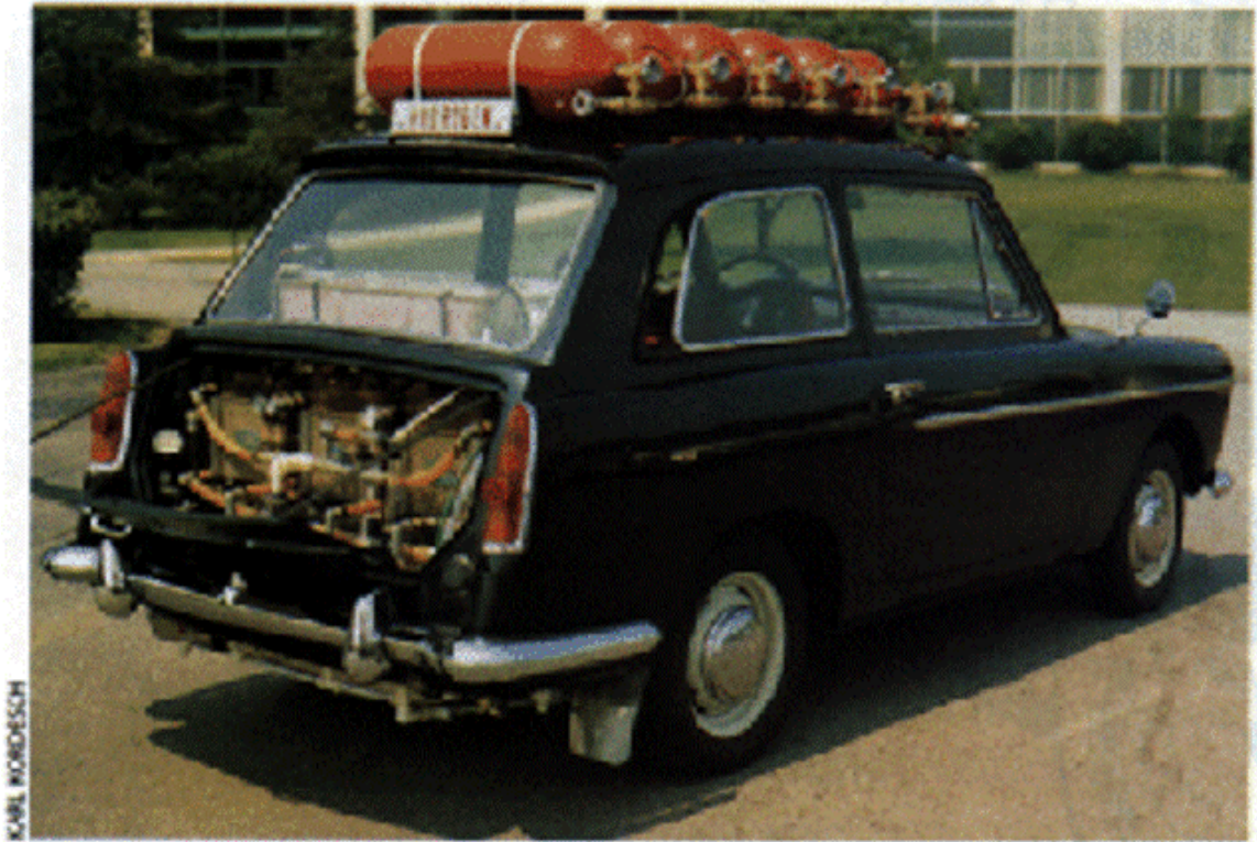
Visible in the 'boot' (trunk) is the fuel cell installation and the six roof-mounted hydrogen tanks. Illustration courtesy of the Union Carbide Corporation.
